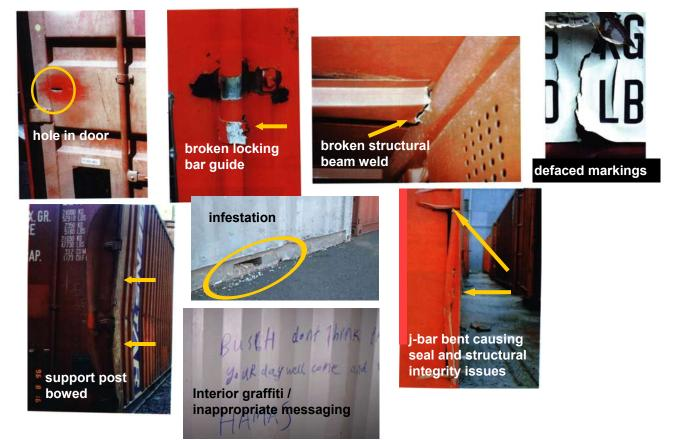
Cargo container doors should seal completely and securely when shut. The container should be light-tight, which will also prevent entry of any external elements into the container while in transit. To ensure a satisfactory light-tight seal, you can conduct a light test by observing the seal performance from inside a closed container. In addition, all door locking hardware (hasps, hinges, handles, bars, bolts, etc.) must be tested and be in good working order *(see below diagram)*.
